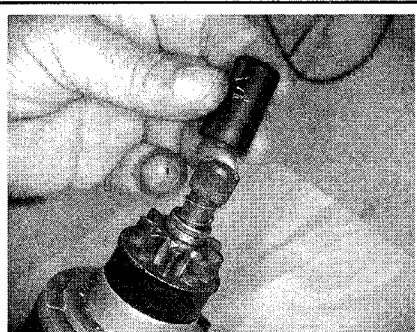
Fig. 198 To disassemble a typical Johnson/Evinrude starter, begin by removing the protective cap. . .
