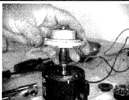
Fig. 205 . . . then remove the end caps (commutator and drive, the drive end cap is shown)
