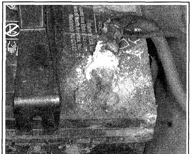
Fig. 120 Ignoring a battery (and corrosion) to this extent is asking for it to fail
