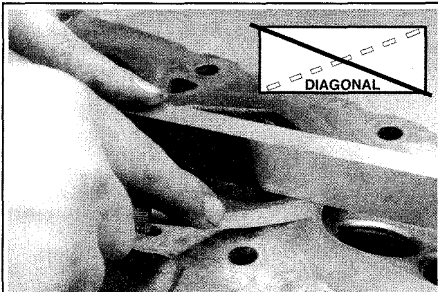
Fig. 118 . . . and at diagonals across the head to be sure the surface is within specification for reuse
