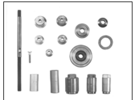
Pinion bearing remover and installer kit P/N 391257 (Use with centering guide from kit P/N 5000009)
