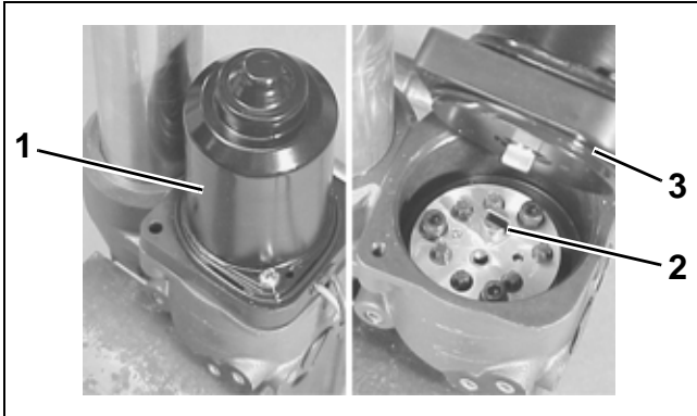
1. PTT motor 2. Drive joint 3. O-ring 001921
