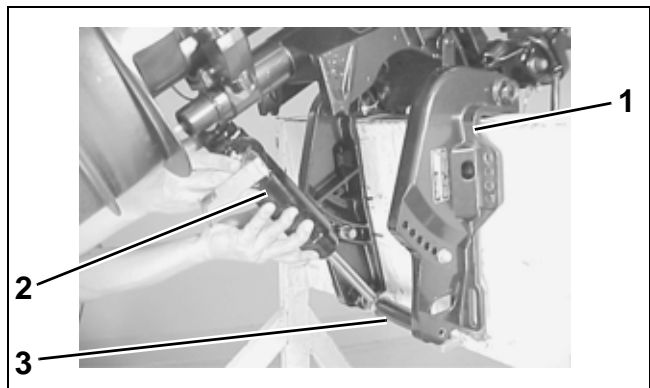
1. Starboard stern bracket 2. Tilt assist cylinder 3. Lower shaft
