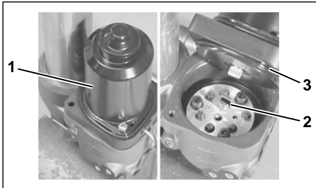
1. PTT motor 2. Drive joint 3. O-ring 001921
