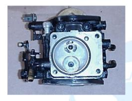
1.8 (Below) Remove the o-ring seal, and pull out the fuel filter.
