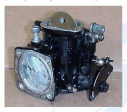
2.2 (Below) Remove all gasket material from all mating surfaces. Some require scraping with a razor knife. NOTE: Use of chemical gasket remover will, in most cases, also remove the paint from the parts being serviced. Any paint removed must be replaced or you risk oxidation.
