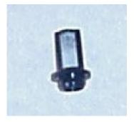
2.5 (Above) Inspect the fuel filter. Use compressed air to blow any sediment back through the filter. If the filter is clogged enough that debris will not release, replace the filter. NOTE: Do not use carb cleaner to try to clean the filters – damage to the plastic may occur.
