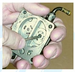
2.4 (Below) Inspect the high and low speed screws for wear and damage. The tips should have a smooth even chamfer without any mushrooming of the tips.
