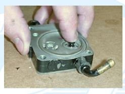
3.2 (Below) When assembling a pump assembly, you will have a choice of three gaskets. One type is for 38mm carbs, the other is for anything above. Of the latter type, there are two choices — one has a slightly different cut-out shape. Make sure you match the new gasket to the old one correctly.
