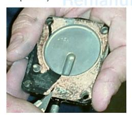
2.3 (Below) Use the tip of a screw driver to push the rubber check valves through the pump body.
