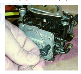
3.5 Re-assemble the pump assembly and regulator chamber covers. Use Medium Strength Loctite (Blue) on all external screws.
