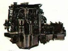
55 horsepower four cylinder in-line valve-in-head 67.6 cu. in. 2.75" bore; 2.83" stroke 8.5:1 compression ratio 5 main bearings mechanical valve lifters maximum rpm: 5000 one 2-barrel carburetor regular gasoline lefthand rotation only 12 volt, 32 amp alternator complete instrumentation closed cooling system dual bronze sea-water pump (use extra pump as bilge pump or
